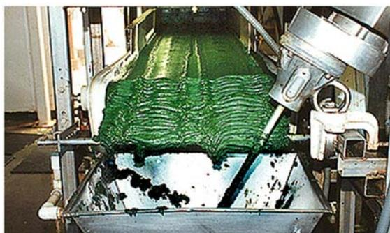
Fig. 5. Microalgal biomass recovered from the culture broth by filtration moves along a conveyor belt at Cyanotech Corporation ([www.cyanotech.com](http://www.cyanotech.com)), Hawaii, USA. Photograph by Terry Luke. Courtesy of Honolulu Star-Bulletin.
