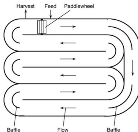
Fig. 1. Aerial view of a raceway pond.
