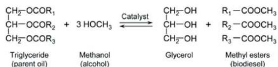
Fig. B1. Transesterification of oil to biodiesel. R<sub>1–3</sub> are hydrocarbon groups.
